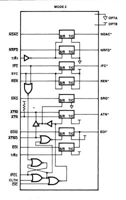
Figure 5. Talker/Listener/Controller Control Configuration
